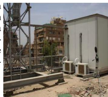
Picture (4-1) Noise measuring at mobile BTSs
