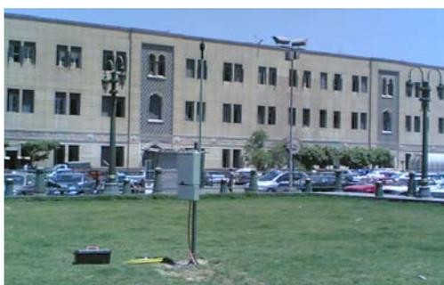
Picture (4-8) Noise Monitoring Station at Ramses Square
