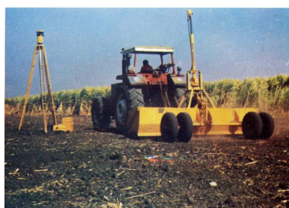
Pic.( 9-3) Laser leveling, deep plowing to improve productivity of degraded land
