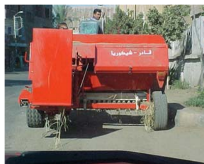
Pressing rice straw using MSEA press machines
