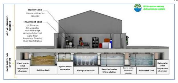
Figure 2-17 Scheme of principle of water recycling
