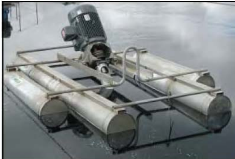
Figure 11: Typical Float Mounted Aerato
