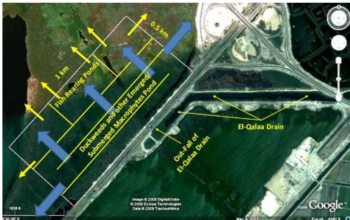
Figure 4: Preliminary Layout of the Proposed In-Lake Engineering Wetland
