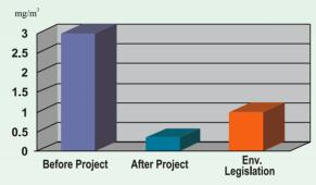
These measurements are in accordance with the limits stated in Law 4/1994, and with the technical agreement with EEAA. Acid fugitive vapors concentration in the work environment were reduced by 88% and emission load to the environment by 95%.
