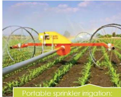
Portable sprinkler irrigation: -Hand-mover lateral -Side-roll lateral
