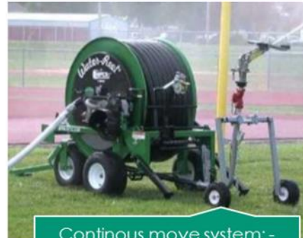
Continous move system: - Center pivot -Travelling gun
