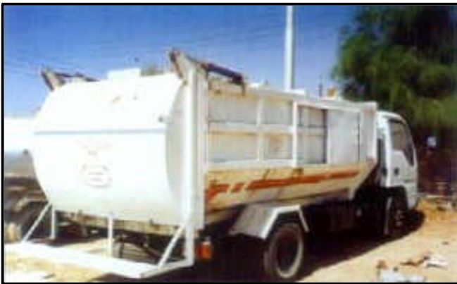
8 ton Isuzu Truck Used to Collect Waste from Industrial, Residential and Commercial Areas
