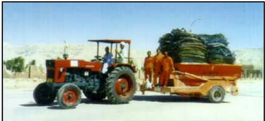
Tractor-Trailer-Container System Used to Collect Waste from Factories
