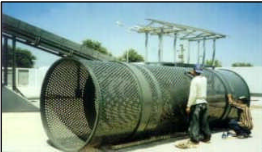
Rotary Screen Used for Sieving Material and Fabricated Locally
