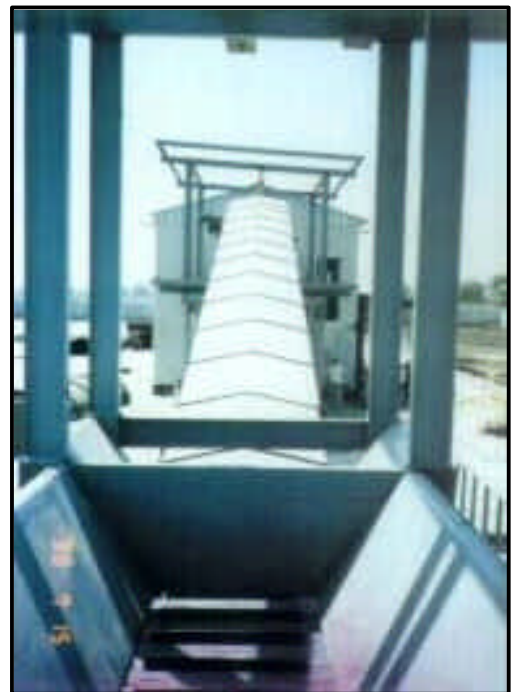
Receiving Hopper and Slat Conveyer Leading to 30mm Rotary Screen and Picking Belt
