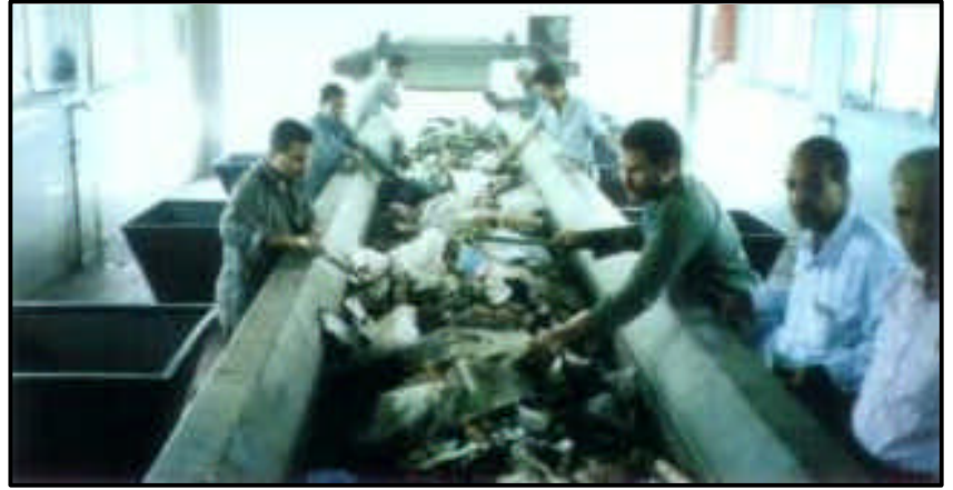
Picking Belt and Sorters Recovering Dry Recyclables
