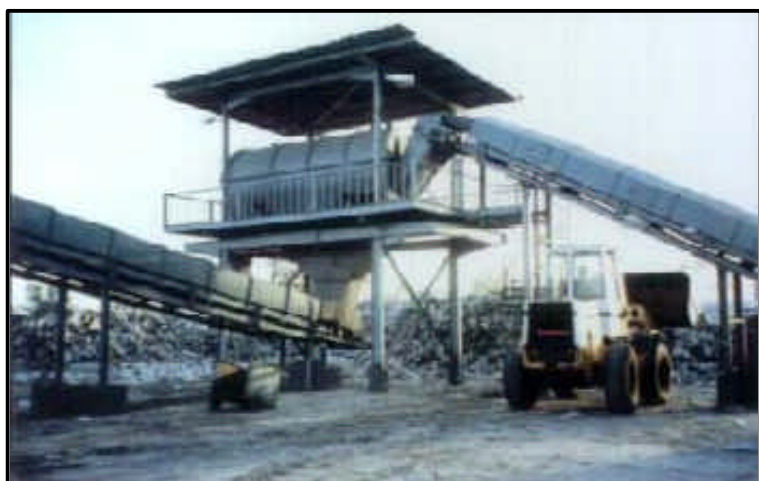
High Level 50mm Rotary Screen and Plus 50mm Rejects area
