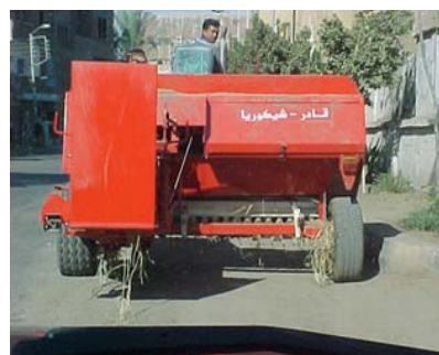
Pressing rice straw using MSEA press machines
